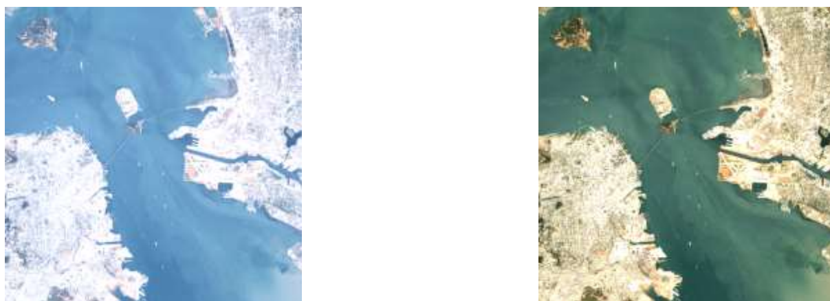
Figure 1-1 Example of LEDAPS atmospheric correction. Left, Top of Atmosphere (TOA) Reflectance composite (Bands 3,2,1) for Landsat-7 ETM+ image of San Francisco Bay (July 7, 1999); Right, Surface Reflectance composite. Both images are linearly scaled from p = 0.0 to 0.15 .
