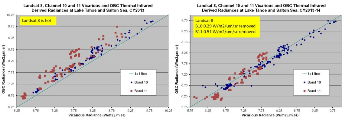
Figure 1: Thermal band errors (left graph) prior to calibration adjustment and (right graph) after calibration adjustment
