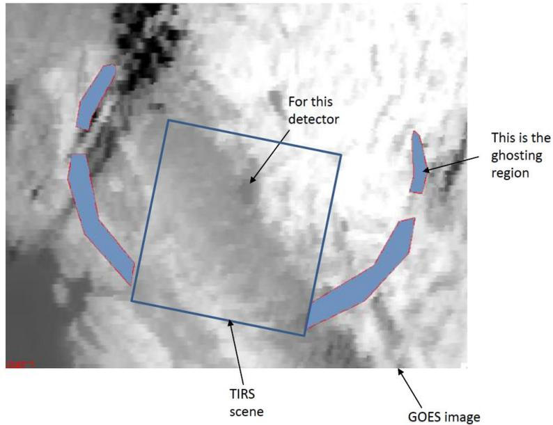
Figure 4: Rough approximation of the out-of-scene contribution to the stray light for a single detector sample
