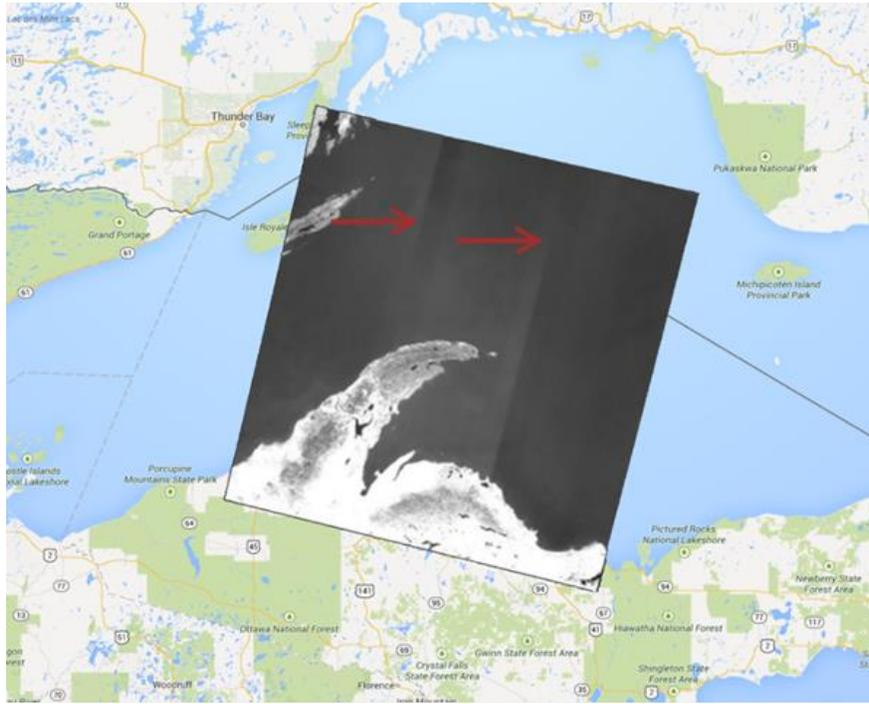
Figure 2: TIRS image of Lake Superior showing apparent time-varying errors
