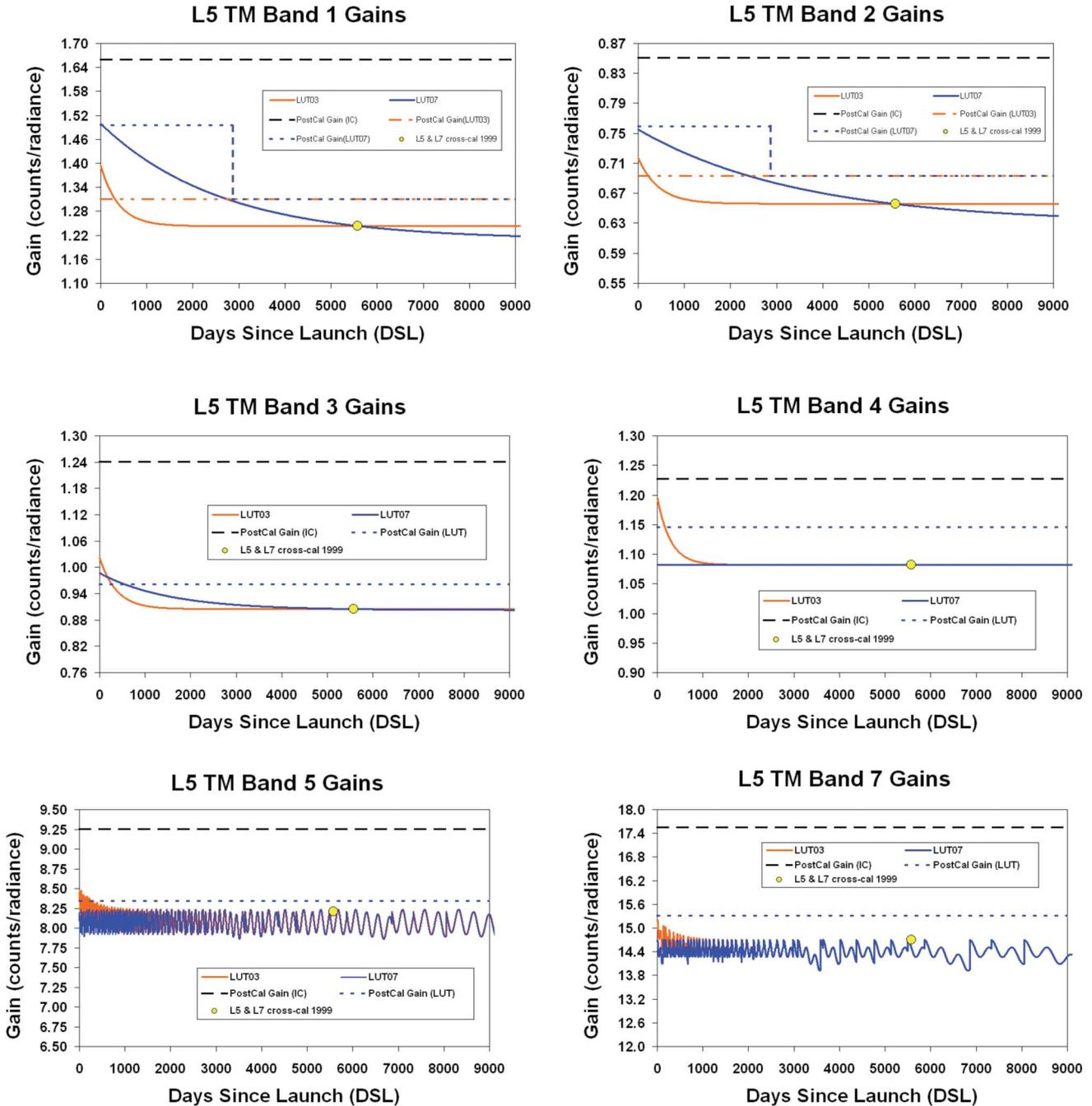
Fig. 1. Lifetime band-average gains implemented in 2003 (LUT03) and 2007 (LUT07) for the L5 TM reflective bands, including postcalibration gains.
